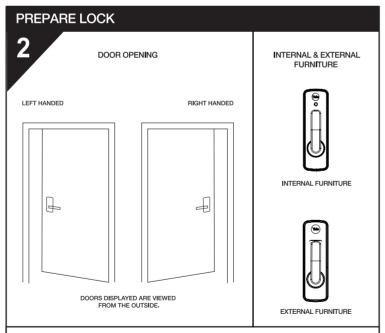
To prepare the lock for install, you will need to establish whether the door is right or left hand opening according to the image above
