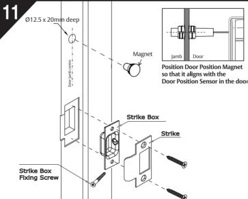
Align the DPS location onto the door jam using a pencil. Drill a 12.5mm dia x 20mm deep hole using the 12.5mm drill bit. Fit the DPS magnet into the door jam. Partially close the door and mark the position of the latch bolt to determine the striker height. Mark and mortice the door jamb to suit the strike box and strike plate. Fix the strike box to the jam and then secure the strike plate over with the timber fixing screws.
