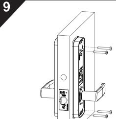
Taking care not to pinch the cables, fit the external lock body to the door.
